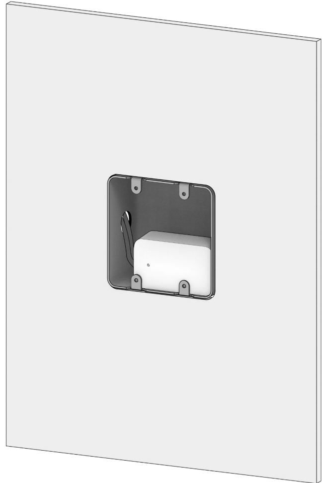
Placing inside a junction box
