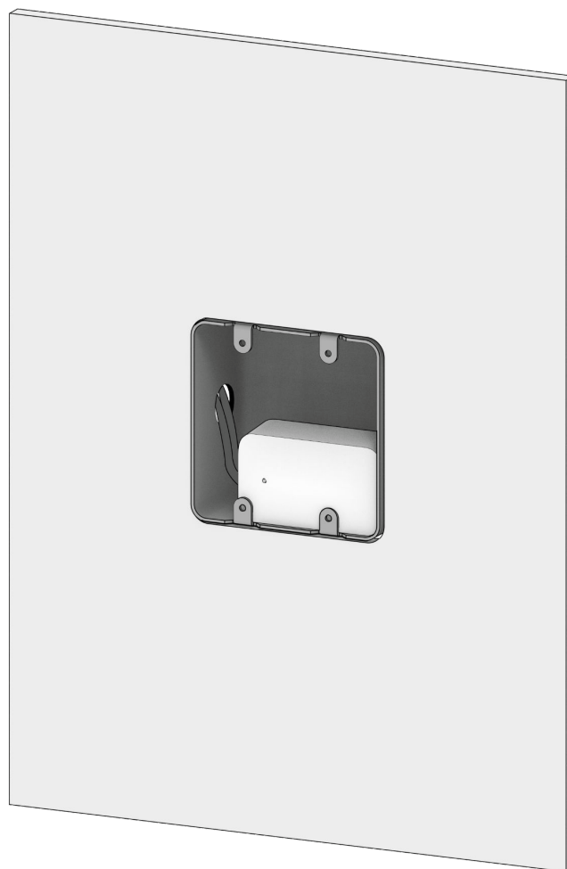
Placing inside a junction box
