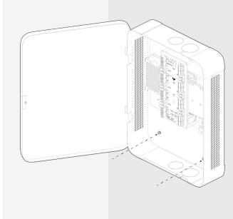
Place the sheet metal enclosure over and onto the mounting plate tabs.
