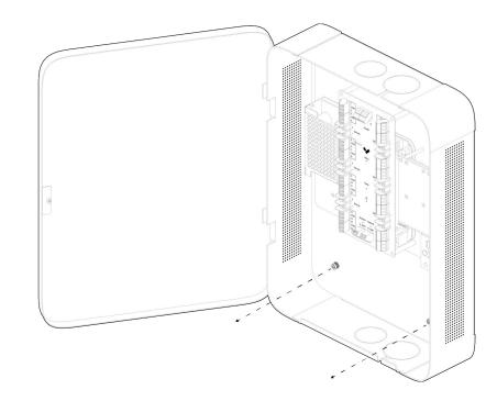
Once the security screws are fully removed, slide the wall mount down and away from the main enclosure.
